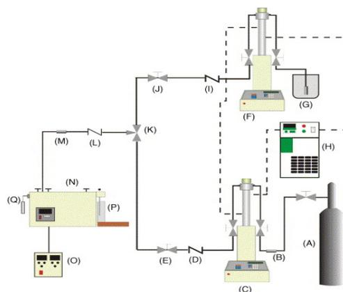
**Figure 18:** Schematic of the supercritical extraction (SC-CO<sub>2</sub>) apparatus
