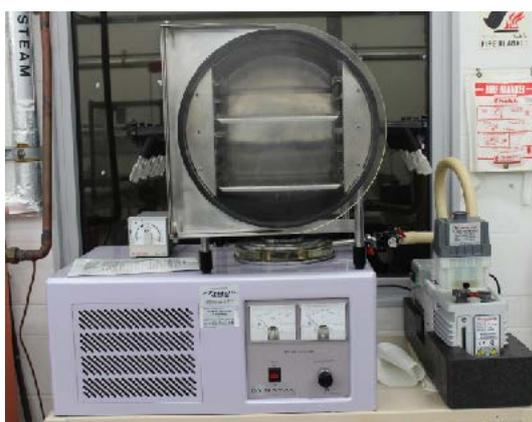
**Figure 16:** Freeze dryer (FD3 Dynavac).
