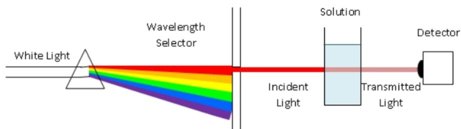
**Figure 10:** The mechanism for spectrophotometry measurement.
