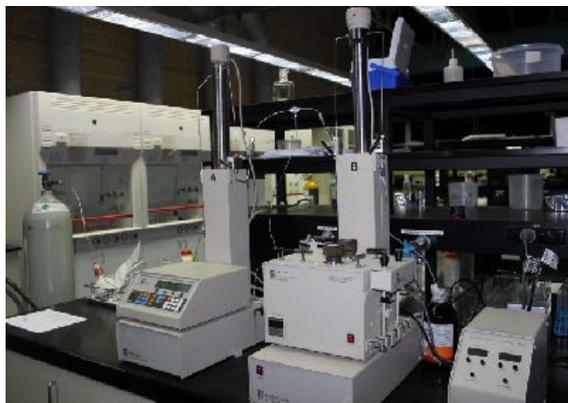
**Figure 17:** Supercritical fluid extraction system.
