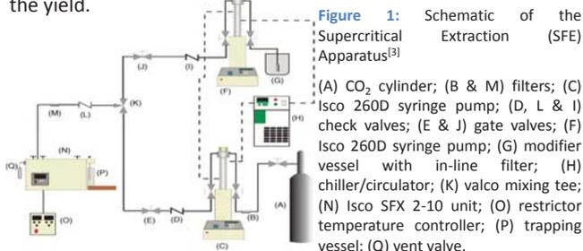
Figure 1: Schematic of the Supercritical Extraction (SFE) Apparatus<sup>[3]</sup>
