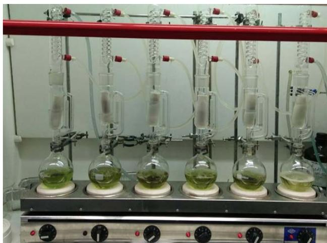
**Figure 21:** Soxhlet system for the extraction of Gac seed oil.
